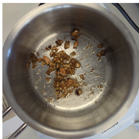
Figure 1: Making iron-gall ink: Frying crushed gall nuts
